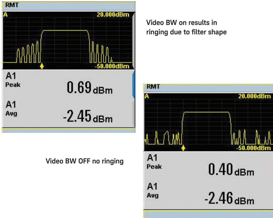
Figure 12. Effects of VBW on power meter measurements of a radar with fast-rising pulse edge.
